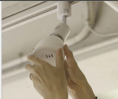
Below The Pi-powered sensor that necessitated the creation of the Pi Zero cluster board. It attaches to standard light fittings
