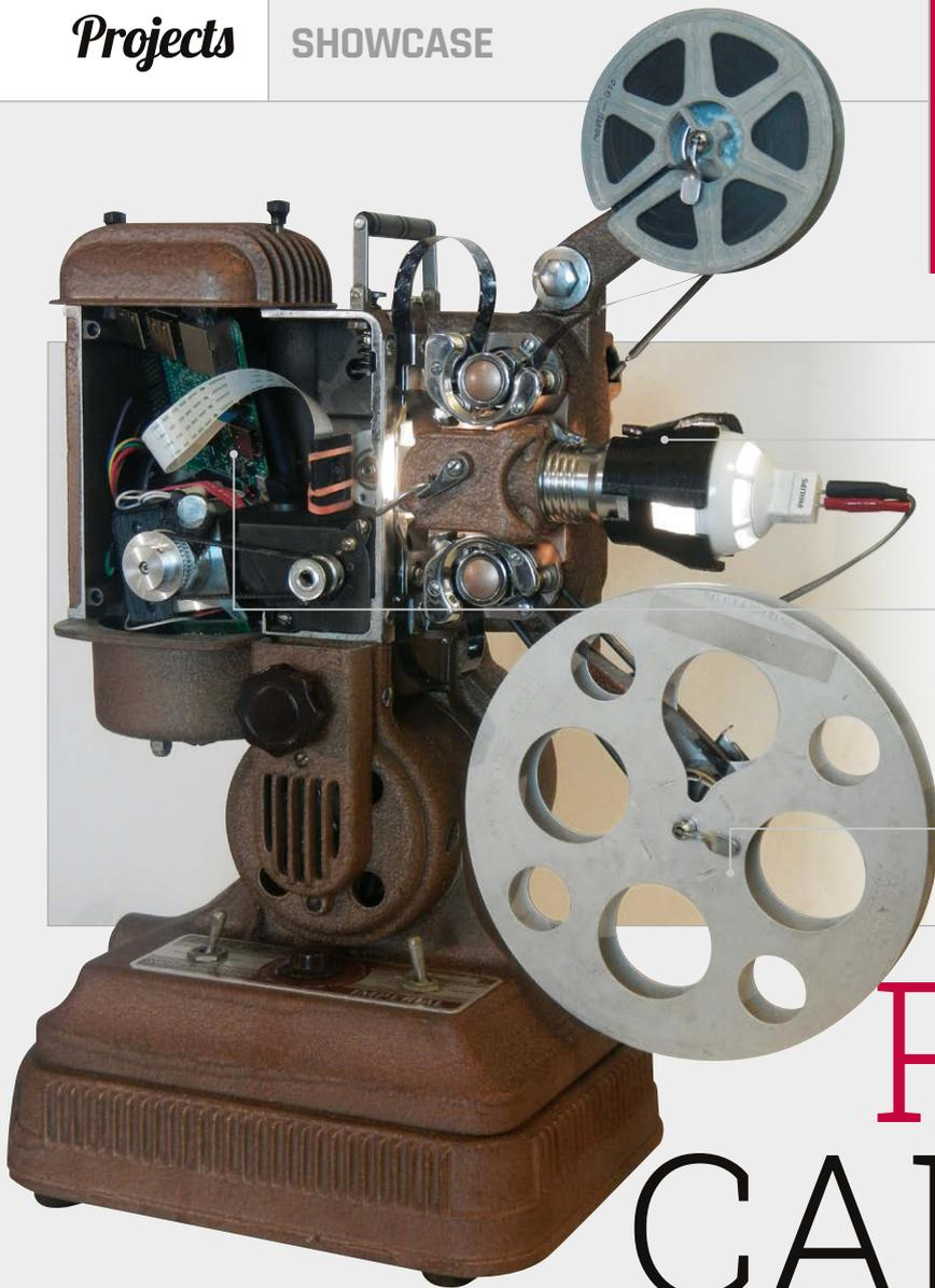
Placed inside the projector, the Raspberry Pi Camera Module records each image, one shot at a time
