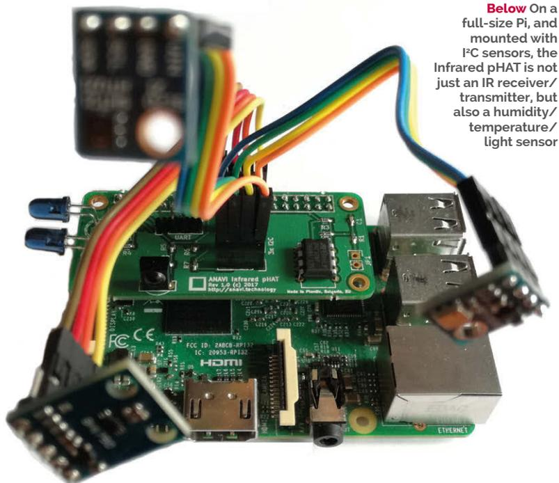
**Below** On a full-size Pi, and mounted with I<sup>2</sup>C sensors, the Infrared pHAT is not just an IR receiver/transmitter, but also a humidity/temperature/light sensor
