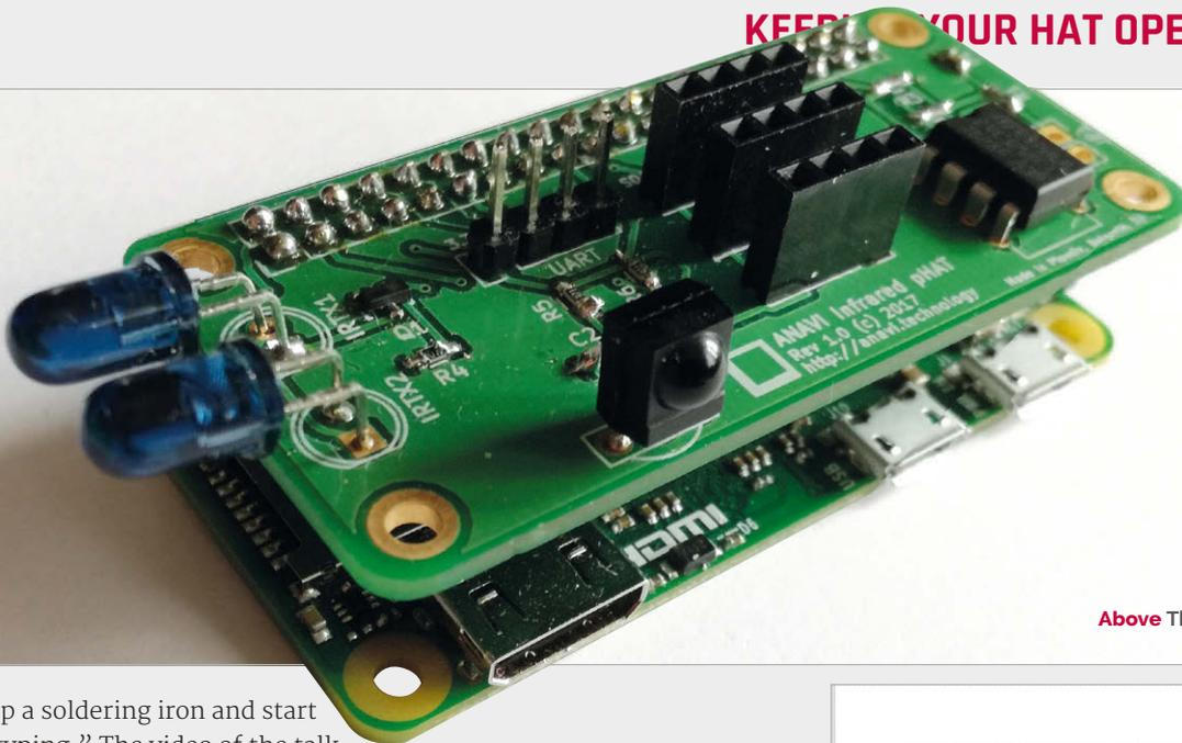
Above The Infrared pHAT in its natural home, on a Raspberry Pi Zero
