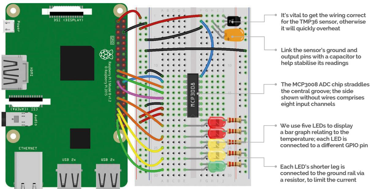
you, the left-hand leg is for power, so connect this to the '+' power rail. The right-hand leg is connected to the '-' ground rail. Its middle leg is the output; here we're connecting to channel 7 (the nearest one) of the MCP3008. Finally, to help stabilise the readings which might otherwise be erratic, we'll add a capacitor to link its output and ground legs.
