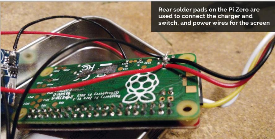
Rear solder pads on the Pi Zero are used to connect the charger and switch, and power wires for the screen
