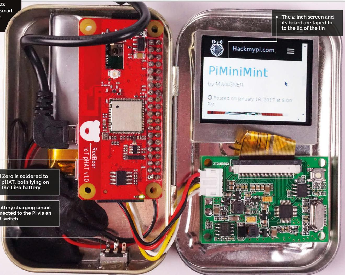
The Pi Zero is soldered to an IoT pHAT, both lying on top of the LiPo battery
