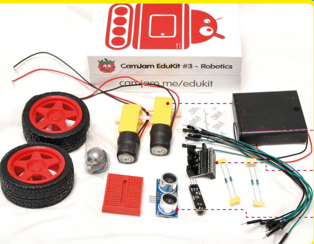
○ These two yellow motors power the red wheels and are used to move the robot around
