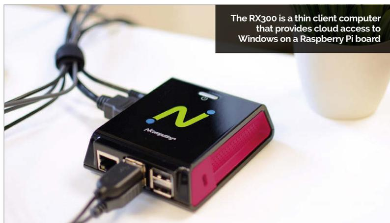
The RX300 is a thin client computer that provides cloud access to Windows on a Raspberry Pi board
