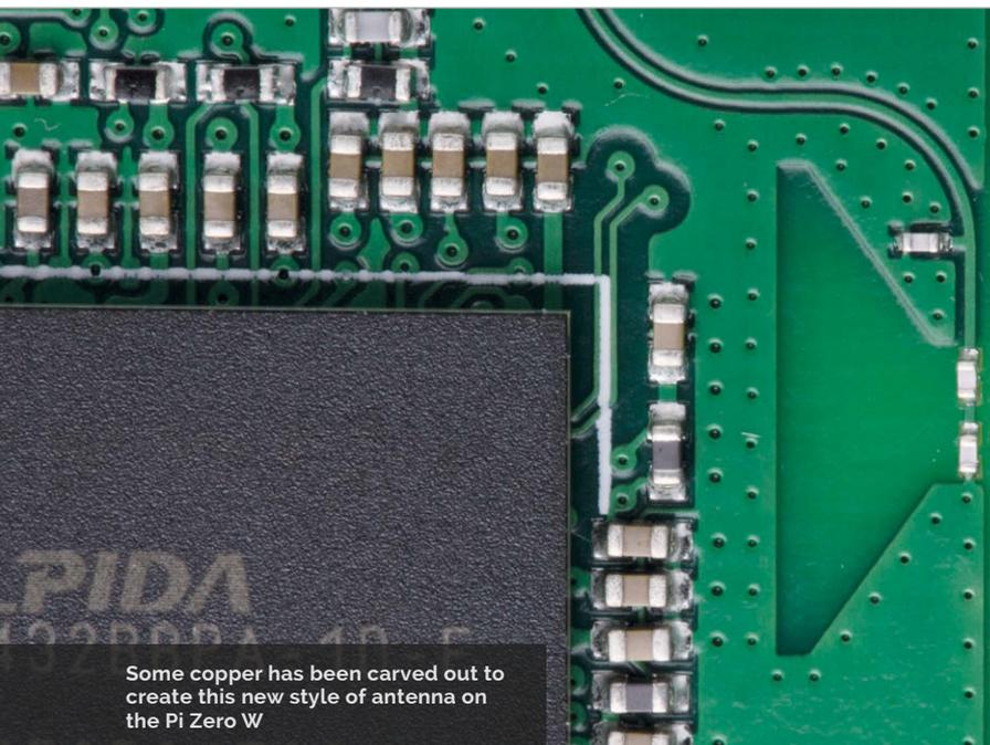
Some copper has been carved out to create this new style of antenna on the Pi Zero W
