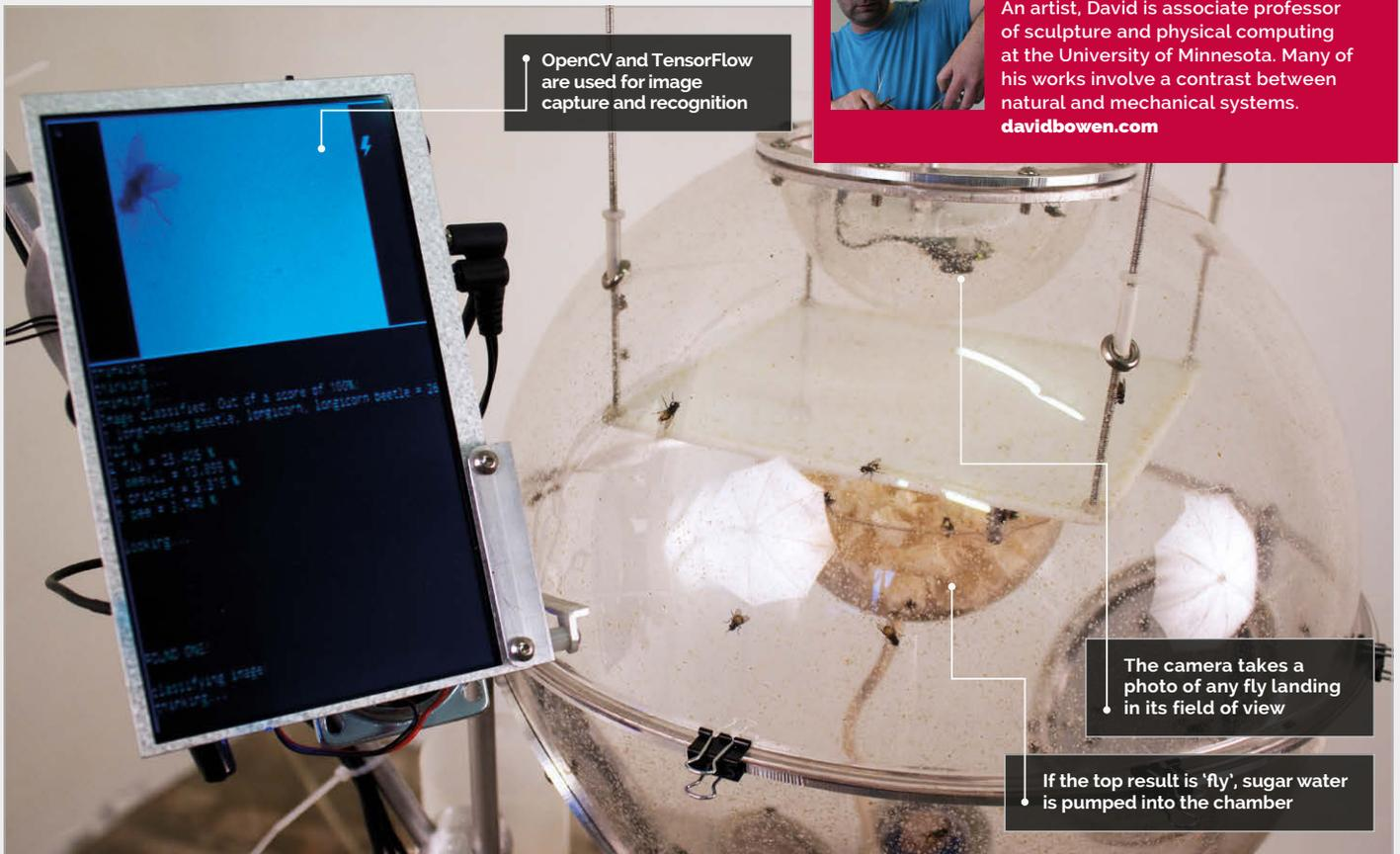
OpenCV and TensorFlow are used for image capture and recognition
