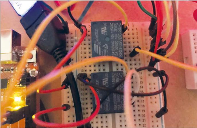
**Above** The coil connectors of the relay are connected to 5V and output on the Explorer HAT Pro. The switch connectors are connected to digital input 1 (and 2 for the second relay) and the ground on the Arduino
