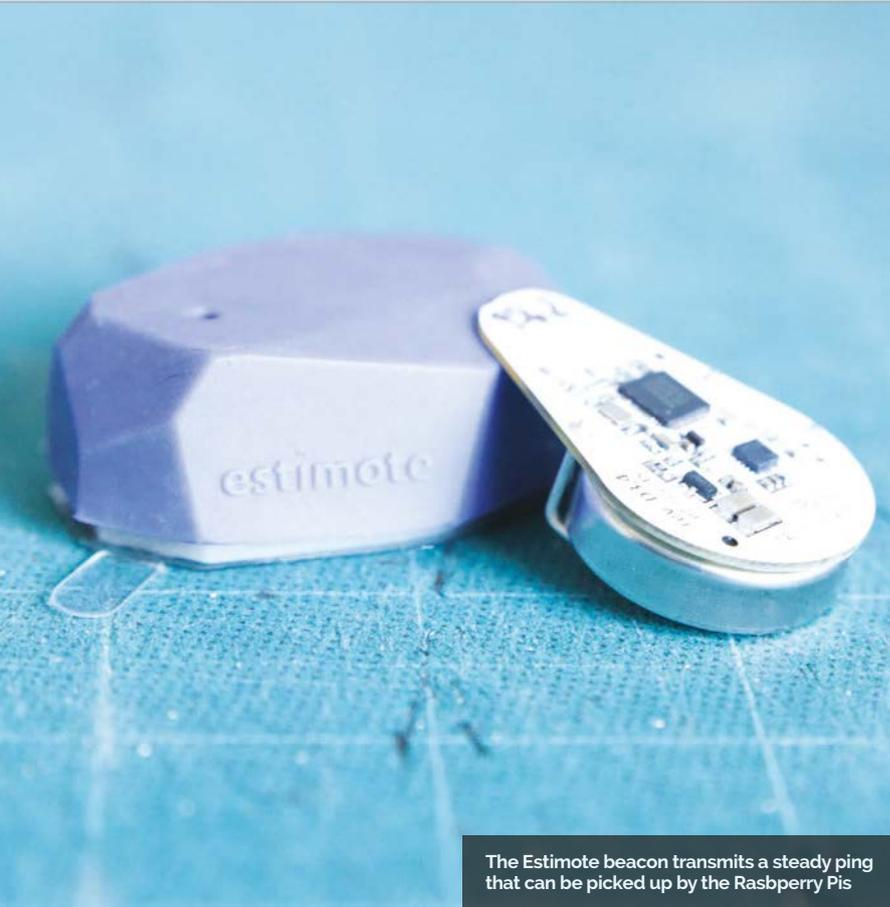
The Estimote beacon transmits a steady ping that can be picked up by the Raspberry Pi
