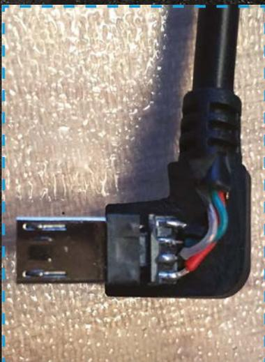
the future, we've decided to take the less invasive route of ripping up a separate micro USB cable and soldering that to the PowerBoost instead.
