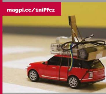
People have made automatons in terms of robots with the Raspberry Pi, but never a fully fledged self-driving car... albeit one on the small side. The technique is roughly the same, though: ultrasonic distance sensors, a camera, and some code to control the car. Read up on how Zheng Wang made one on his blog via the link.
