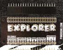
sensors – we've seen Explorers used in robots due to this. It allows for analogue inputs as well as other inputs and outputs, and has its own Python library for quick development. Great for tiny projects.
