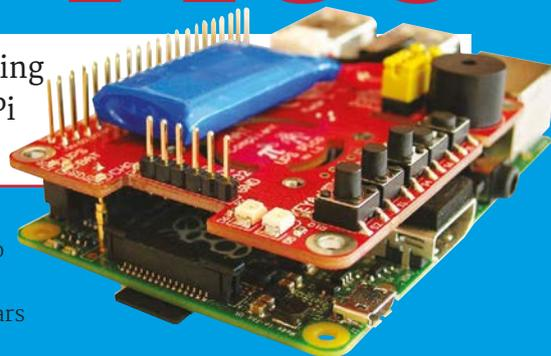
cut; the advanced model will keep it up and running for eight hours then shut it down safely. It keeps itself charged up via the GPIO pins, and an embedded measurement system detects if a power problem has occurred.
