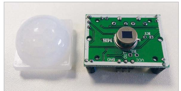
Connect the VCC to the 5V pin, and GND to any ground pin of your Pi, then connect the OUT pin to any GPIO pin. In the diagram below, pin 4 has been used.
