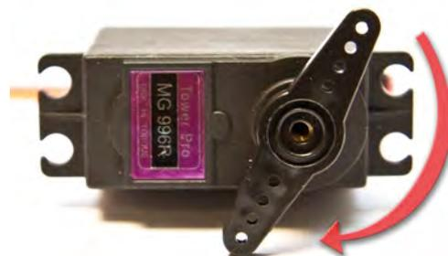
▲ The `setAngle()` function will move the servo armature from its existing position to the new angle
