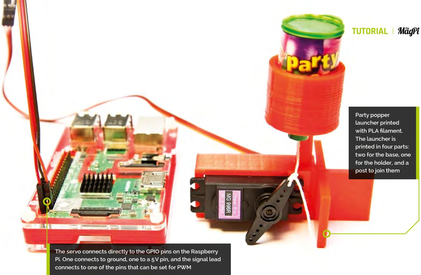
The servo connects directly to the GPIO pins on the Raspberry Pi. One connects to ground, one to a 5V pin, and the signal lead connects to one of the pins that can be set for PWM
